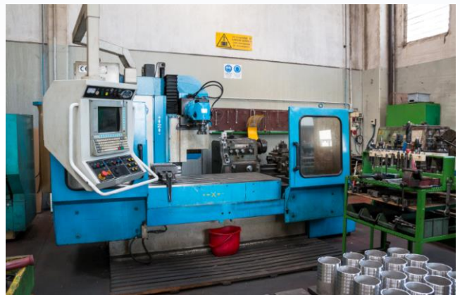
Boring machine “KOMPAKT” Milling fixed worktable Dimensions 2m x1m x1m (h)
