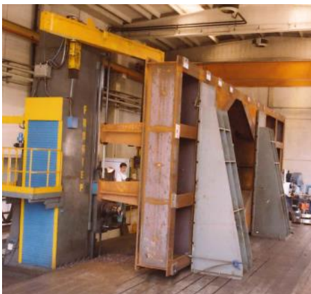
Boring machine “KOMPAKT” Milling fixed worktable Dimensions 2m x1m x1m (h)
